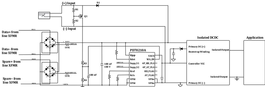
When an external adapter is connected, the PD70210A WA\_EN pin is used for disabling the isolation switch and PSE input power. The WA\_EN resistors divider depends on the WA\_EN threshold of the PD70210A.
