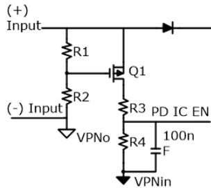
R1 and R2 sets a rough threshold for Pfet Q1 enable to detect whether an external adapter exists or not. It should be set to be a lower threshold than PD70210A disable levels. R3 and R4 set the PD70210A disable threshold. So, in the case of a 36 V–57 V external adapter, the disable setting can be selected as follows:
