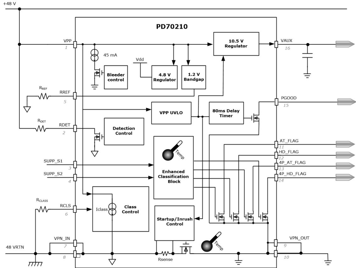
The following illustration shows the functional blocks of the PD70210A/PD70210AL devices.
